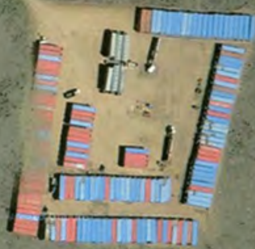
Weld County, northeast of Firestone; Frac tanks hold water/chemicals being prepared to go down a well or that has come out of a well. 166 tanks, each holding 500 barrels/21,000 gallons totals 3.5 million gallons of water.
