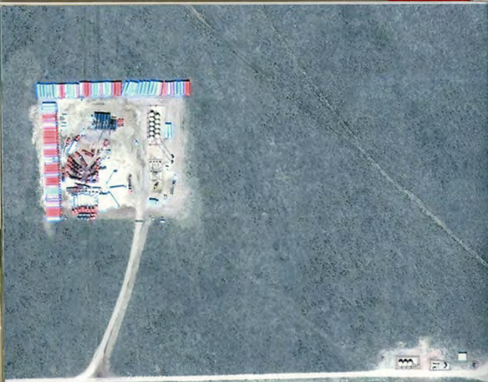
The right well pad has a pool tank, 150 ft. diameter, which holds 42,400 barrels/1,780,590 gallons, and 222 frac tanks contain 4.6 million gallons of water. This site for hydraulic fracturing contains 6.4 million gallons of water.
